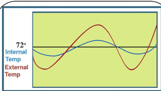
**The effect of thermal mass, as shown above, helps to smooth out large temperature swings. For example, if the temperature outside is hot or cold, or fluctuates dramatically between day and night, the thickness or "mass" of the super insulated ICF wall system helps to delay the transfer of that temperature to the interior of the home.**
